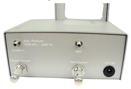
7. Connect the power supply using the included special cable.
